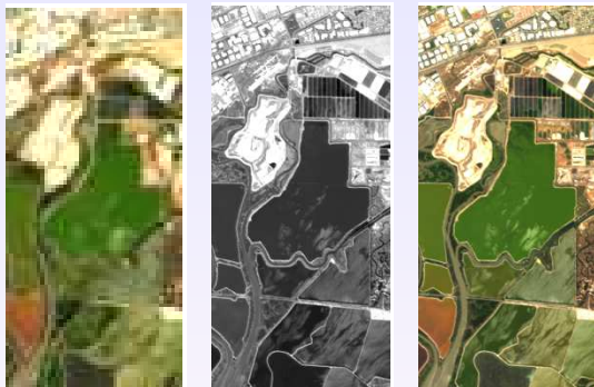
Figure: (a) Hyperspectral Image (size: 99 \times 46 \times 224 , res.: 80\text{m} \times 80\text{m} ) (b) Panchromatic Image (size: 396 \times 184 \times 1 res.: 20\text{m} \times 20\text{m} ) (c) Target (size: 396 \times 184 \times 224 res.: 20\text{m} \times 20\text{m} )
